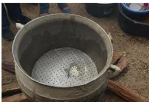
**Figure 5: A False Bottom (Sand Casted) and a Parboiling Pot (Left: FB is inserting in the pot, Right: FB in the pot. A parboiler put paddy on inserted FB)**
