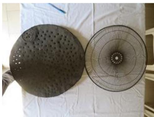
**Figure 7: Petro drum lid (left, good as a false bottom because it resists rust) and Fun cover (Right)**
