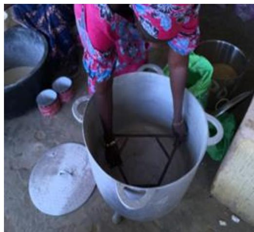
**Figure 8: Left: A Support in the Pot, Right: A False Bottom is on the Support**
